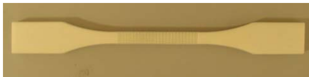
Fig. 2 Specimen used to test the effective modulus of the PA scaffolds in tension
